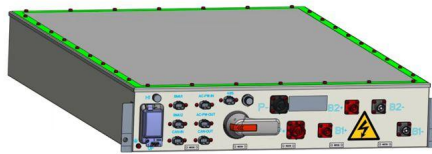
Figure 6 - 4 Schematic diagram of the high-voltage box handle status corresponding to the DC circuit shutdown
