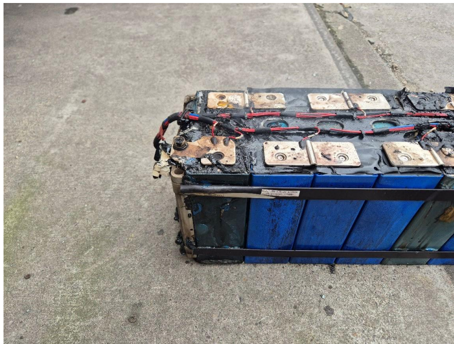
Figure 9 - 280Ah cells after test 1 and 2.
